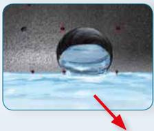
The unique "multicell" tread compound contains microscopic bubbles and tubes which clear water rapidly from between the tyre and ice or snow surface and assure a proper contact of the tyre on the road.
