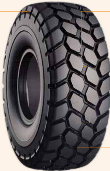
Double-reinforcing tie-bars minimise longitudinal elongation and deformation of the centre blocks upon surface contact. This reduces internal friction, minimises irregular block wear and extends the life of the tyre.
